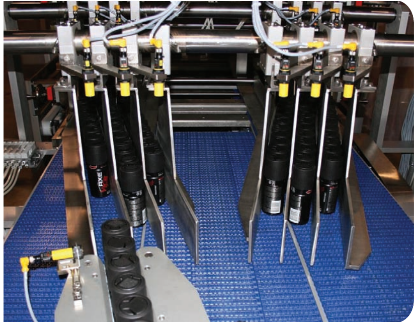
Allen-Bradley Kinetix 6000 servo drives receive products and convey them down to one of six lanes. Multiple lanes increase throughput without sacrificing reliability.
